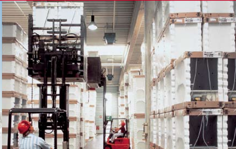
Pressure-resistant packaging made of Styropor® for refrigerators
